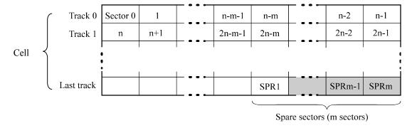
Note: This drive manages alternate spare areas for each cell, which is a set of cylinders. One cell consists of 27 cylinders.
